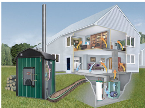
Fig. 2. Hydronic heater integrated with heating system. Shown here is the unit integrated with a forced hot air furnace, but other integrations may include radiant floors, radiators, or baseboards [30].
